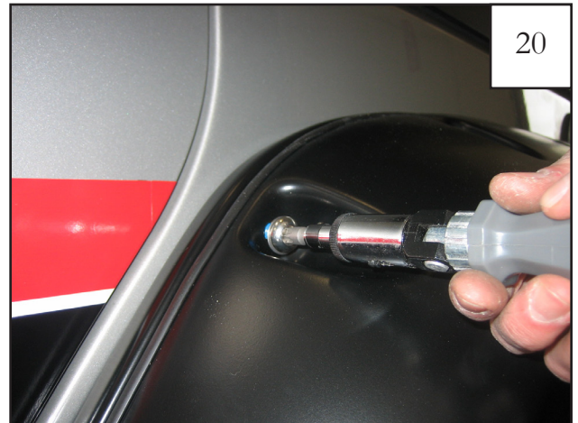
20 Start Screws/Washers through pocket holes in flare and into Threaded Clips installed in Step 11 (8 places) starting at the front and working your way to the back. Do not tighten.
